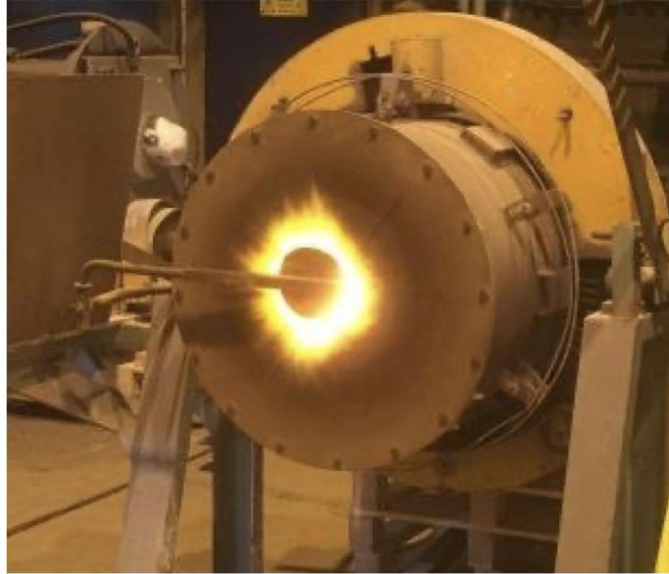
Figure 6. Test configuration of plasma generator from ScanArc together with rotary batch kiln from Cemta Research.
