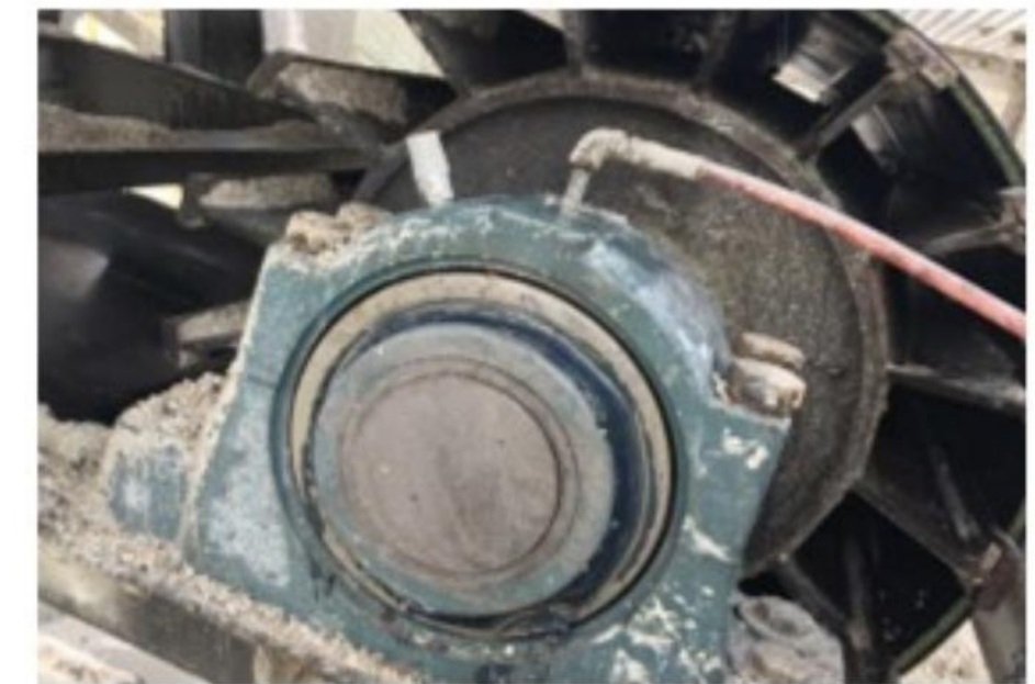
Smart sensors (shown here as the white cylinder on the bearing) allow equipment to be monitored in locations which may be difficult or dangerous to reach.
