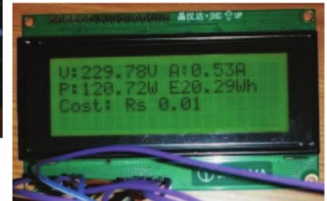
FIGURE 9: OUTPUT VALUES AS DISPLAYED IN LCD
