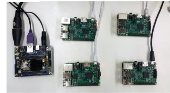
Fig. 6: Embedded computer boards used as controllers.
